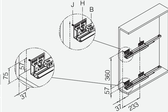
2. Set the basket on the rails, make sure (L) lock the rail, and rail tail lock the basket
