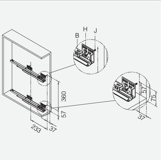
2. Set the basket on the rails, make sure (L) lock the rail, and rail tail lock the basket
